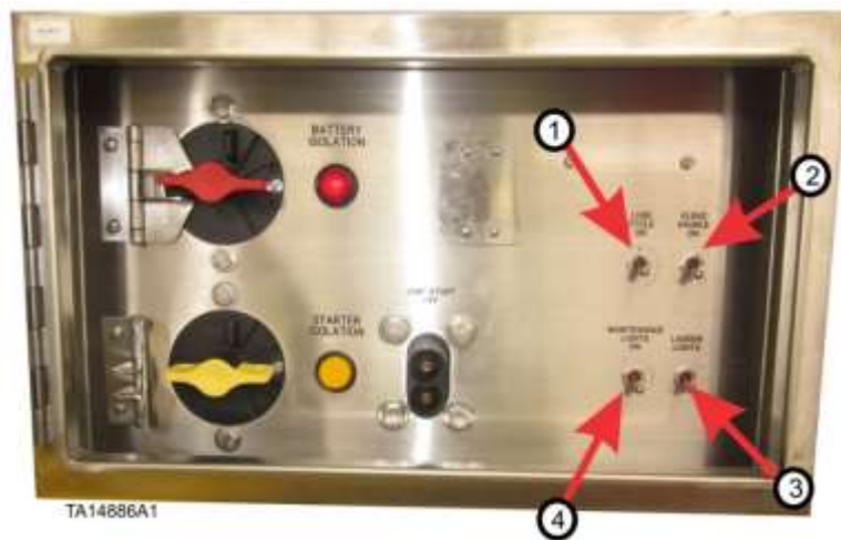
1) Auto lube switch inside 2) KLENZ enable 3) ladder lights 4) maintenance lights Located on left rear of machine
