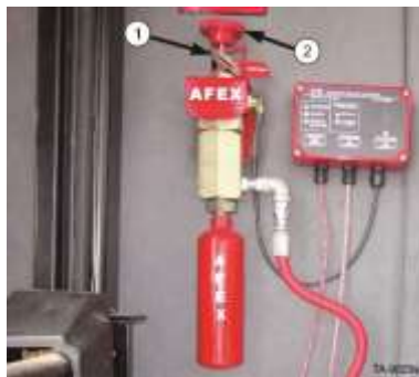
1) Pull pin, 2) Strike knob to actuate fire suppression system AFEX cab mounted firing mechanism with circuit monitoring panel (typical)
