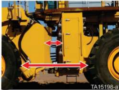
MACHINE STEERED STRAIGHT (Arrows indicate crush hazard areas-present on BOTH sides of machine)
